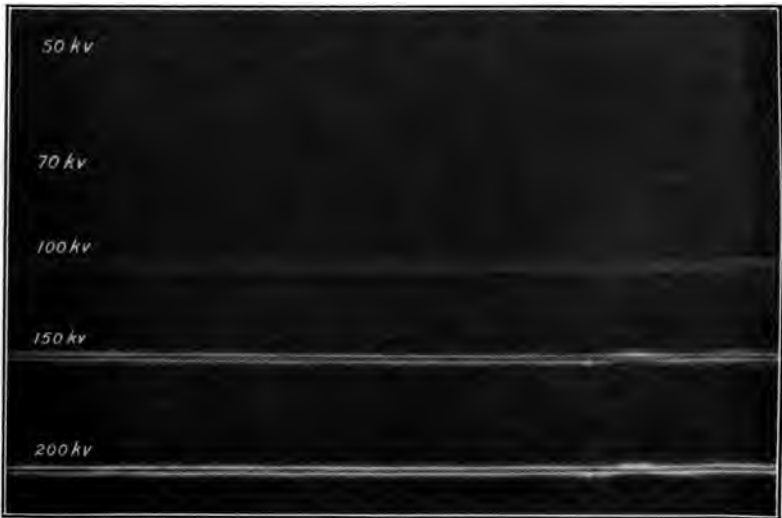
FIG. 62.—Corona on copper wire polished after each exposure. Diameter, 0.186 cm.
